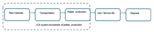
Figure 1. System boundaries of life-cycle assessment. The diagram describes the life-cycle stages of pellets production. LCA excludes the use and end of life life-cycle stages.
